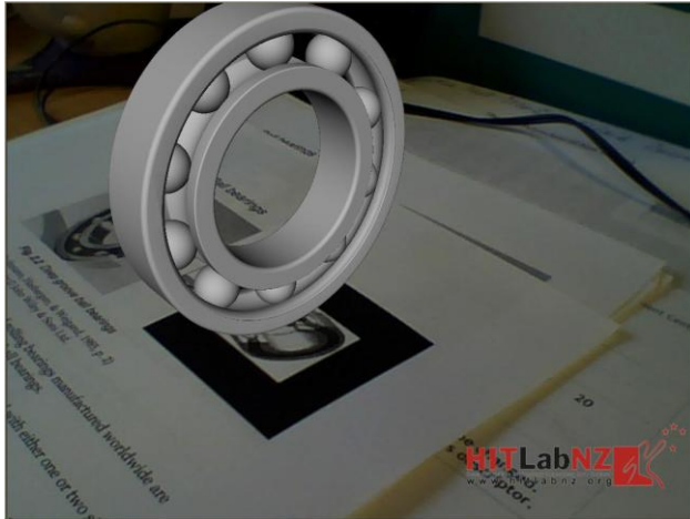
Fig. 1 An image of a roller bearing, viewed on a computer screen via a webcam focused on the augmented reality target
